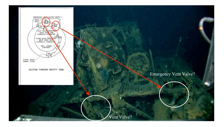
Possible **Safety Tank** Vent Riser, Vent, and Emergency Vent Valves.
