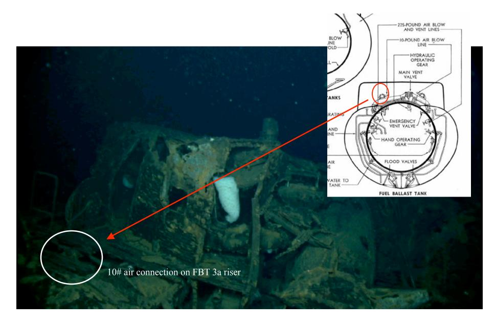
Possible Fuel Ballast Tank 3 Vent Riser and 10# air connection source: attack analysis 2: Open hatch 22
