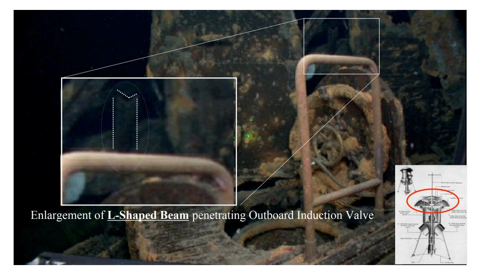
Amidships; starboard side, looking to port; Camera is outboard of open After Battery Hatch source: Attack Analysis 2, open hatch 16, photo#5115765628423339762
