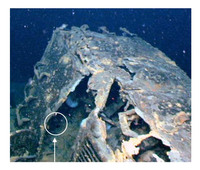
Possible shell damage / hole in deck in aft Conning Tower Fairwater source: Black 04: 01:34:28:16
