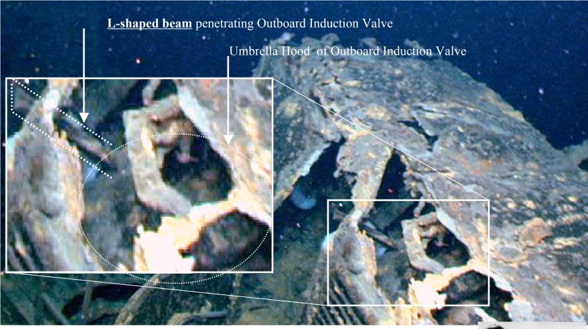
Amidships, starboard side. ROV is on starboard side of Conning Tower Fairwater facing port and aft. Source: Black 04 01:34:28:16
