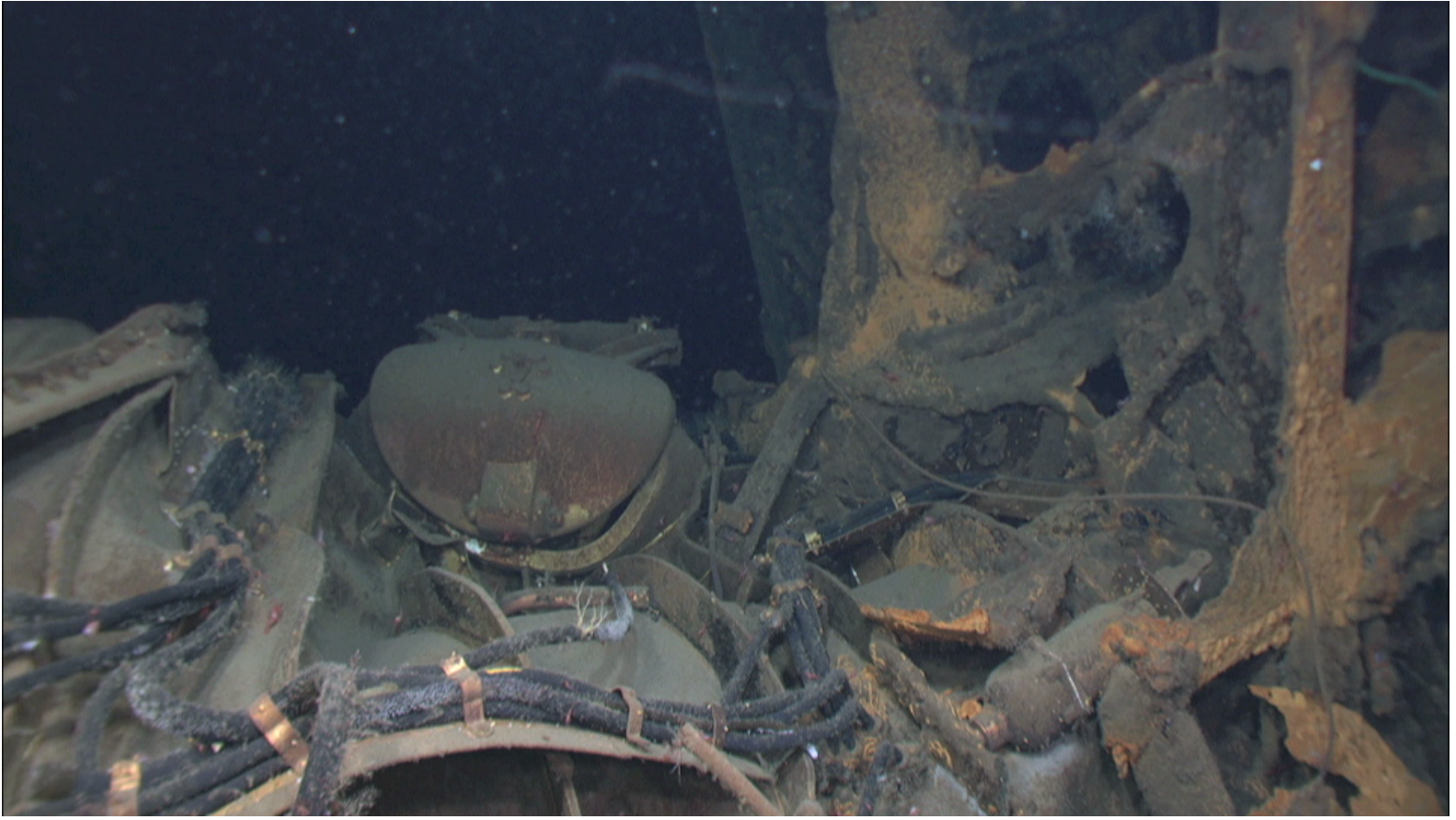
Upper conning tower hatch was bent in a strange manner.
